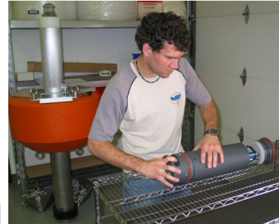
Above: Kevin Rose works on data-logger with buoy in the background. The data logger controls power to the sensors and sampling frequency, stores data, and sends data back to a central server on user defined intervals.
